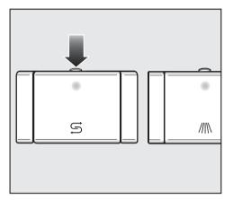
Press the button on the lid of the salt reservoir in the direction of the arrow until the flap springs open.
